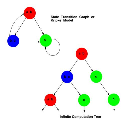
(Unwind State Graph to obtain Infinite Tree)
