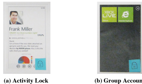
Figure 5. Paper prototypes of the two proposed sharing mechanisms. The blue padlock icon in (a) indicates that the access is limited to a specific e-mail and in (b) that is limited to a specific set of applications.
