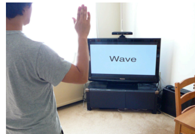
Figure 1. The proposed system can identify users based on 2 seconds of hand waving gesture measured by a Microsoft Kinect.
