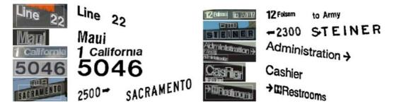
Figure 16. Example of binarization on the detected text.
