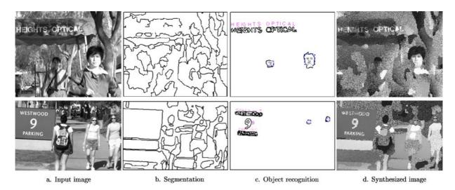
*Figure 17.* Results of segmentation and recognition on two images. The results are improved compare to the purely bottom-up (AdaBoost) results displayed in Fig. 15.
