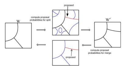
*Figure 11.* An example of the split- merge sub- kernel. State W consists of three regions and proposals are computed for 7 candidate splits. One is selected, see arrow, which changes the state to W'. Conversely, there are 5 candidate merges in state W' and the one selected, see arrow, returns the system to state W.
