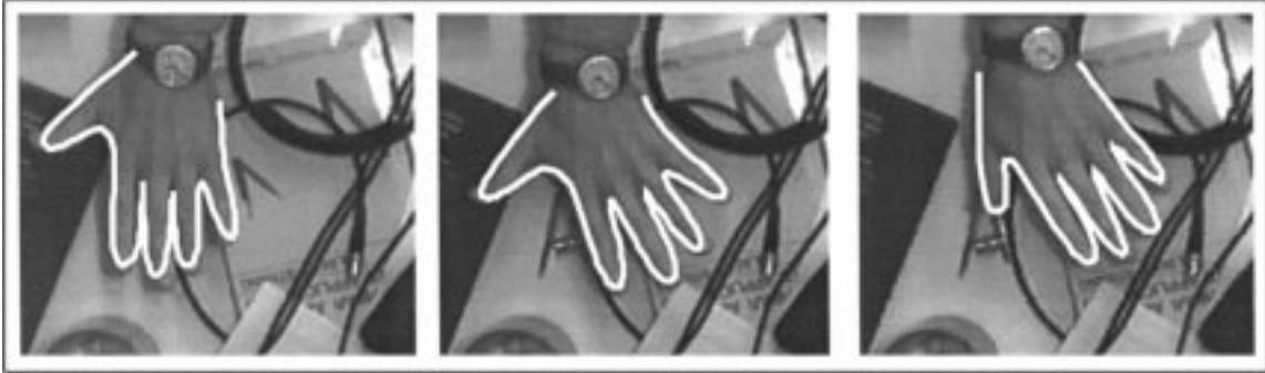
Figure 16. Tracking a flexing hand across a cluttered desk: representative stills from a 500 field (10 s) sequence show a hand moving over a highly cluttered desk scene. The fingers and thumb flex independently, and the hand translates and rotates. Here the CONDENSATION algorithm uses N = 1500 samples per time-step initially, dropping gradually over 4 fields to N = 500 for the tracking of the remainder of the sequence. The mean configuration of the contour is displayed.
