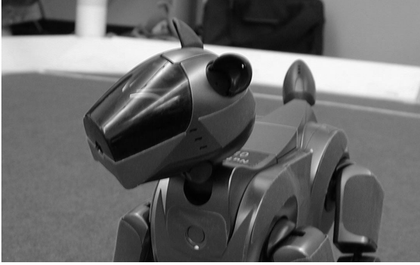
Figure 1: This is one the Sony AIBO robots for which this world model was implemented. The round aperture at the tip of the robot’s nose is the CCD camera that is used to capture visual sensor data.
