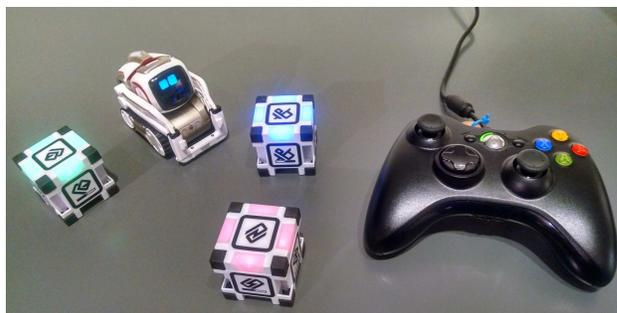
Fig. 1. The Cozmo robot, its three unique light cubes, and the game controller used with Calypso.
