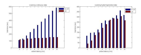
Figure 5: Effects of CNF on the actual system. (a) Scanning large files. (b) Highly fragmented data.
