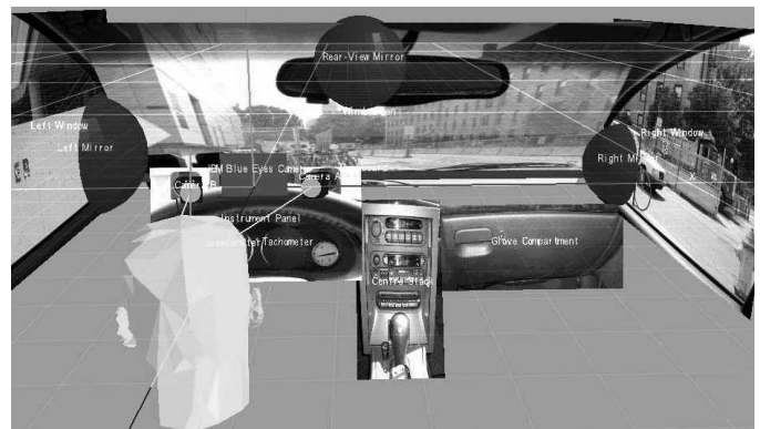
Figure 5. - Cameras track driver's eye position
