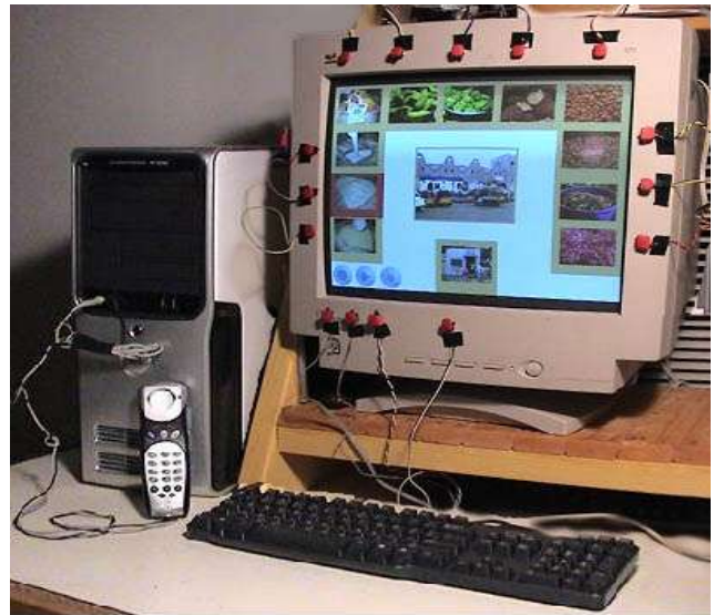
Fig. 11. Tamil Market kiosk prototype. Phone mic and modified keyboard with flex buttons are made from locally available recycled components.
