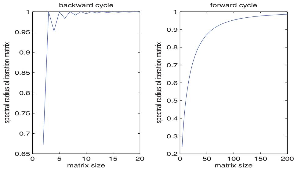
FIG. 6.1. Spectral radius of the SOR iteration matrix for backward (reverse) and forward cycles, where  $\omega = \frac{2}{1+\alpha}$ .
