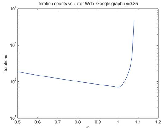
FIG. 6.3. *SOR convergence for the Web-Google matrix: The number of iterations it took to reach a tolerance of  $10^{-10}$  in terms of the  $\ell_1$ -norm of iterate difference for  $\omega = [0.50 : 0.01 : 1.08]$ .*
