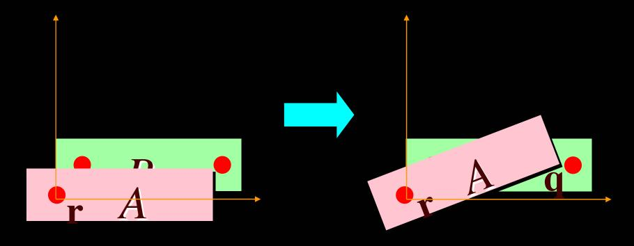
Next, we rotate A by v (the "elbow" angle)
