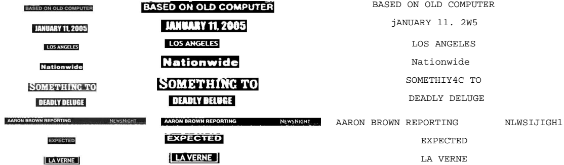
Figure 6. Extracted text lines, corresponding binarized images and text extracted from a commercial OCR
