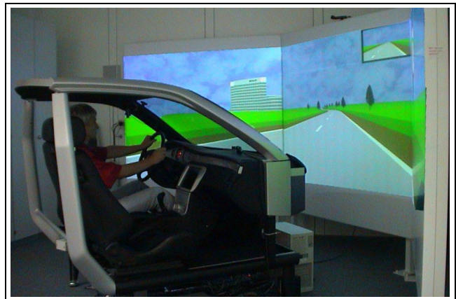
Figure 1: View of the Bosch driving simulator
