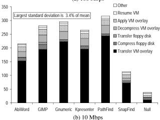
Figure 3: Startup Delay in Seconds
