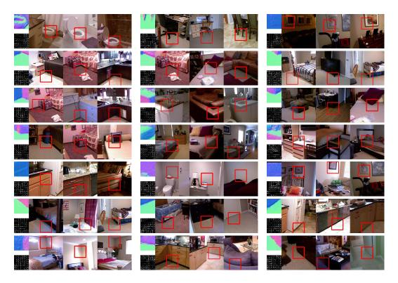
Figure 4.2: Example primitives discovered by our approach. (Left: canonical normals and detectors; right: patch instances). Our discovery method finds a wide range of primitives: **Row 1:** objects and parts, **Rows 2-4:** 3 and more plane primitives, **Row 5:** 1 plane, **Row 6-7:** 2 planes. Our primitives contain visual synonyms, (e.g., row 6), in which different appearance corresponds to the same underlying geometry.
