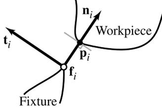
Figure 2: A local frame attached to fixel  $i$ .
