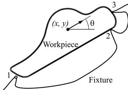
Figure 1: A workpiece nearly seated in a fixture.
