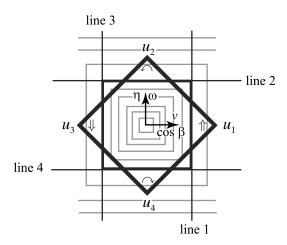
Figure 5: Geometric construction of level sets of the Hamiltonian for the differential drive.
