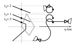
Figure 7: Some level sets of the Hamiltonian and corresponding extremals for a differential drive pushing a block.
