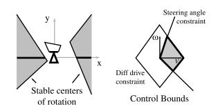
Figure 4: Quasistatically stable rotation centers and control bounds for a differential drive pushing a block.
