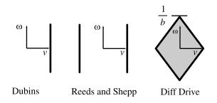
Figure 2: Control regions for steered cars and differential drives.
