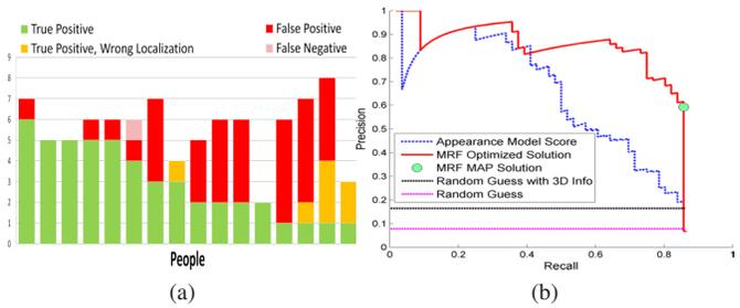
Figure 10: Dataset 3: (a) Results for individual people. The last two bars correspond to the cases where the 3D localization failed. (b) Precision-recall curves.
