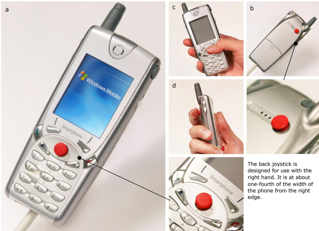
**Figure 1a.** front view. Almost all of the original phone components are preserved. The LCD screen is fully functional. The two joysticks communicate with a computer through a PS/2 connection using the cable at the bottom of the phone.
