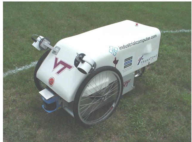
Figure 1. Navigator – a 3-wheeled differentially driven autonomous vehicle
