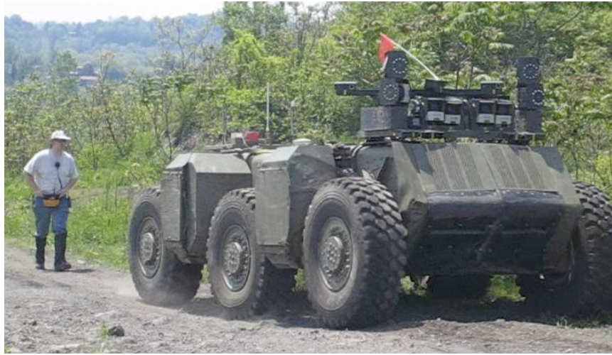
Figure 8.2: The Maximum Margin Planning (MMP) algorithm [3, 104] learns cost functions that make behavior demonstrated by experts optimal to the planning algorithm used by a robot. In the above image, an experienced driver is teleoperating a mobile robot and providing an example of the driver’s preference for driving on roads. This and other demonstrations were used by MMP to learn a cost function for the local perception system of the robot which imitated the expert’s behavior, and outperformed an engineered cost function that had been developed through extensive field testing and parameter tuning [21, 24].
