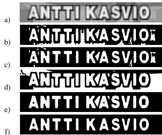
Fig. 3. Applying grayscale consistency : a) original image b) text layer (GEM K=3 ) c) same as b), after the connected component analysis d) text layer (Otsu), e) same as d), after the connected component analysis, f) same as c), after the gray level consistency step.
