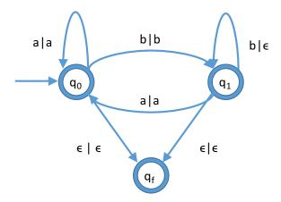
We would like to represent the transducer as a process T that receives the input string, symbol by symbol, from the left and sends the output string, again symbol by symbol, to the right.
