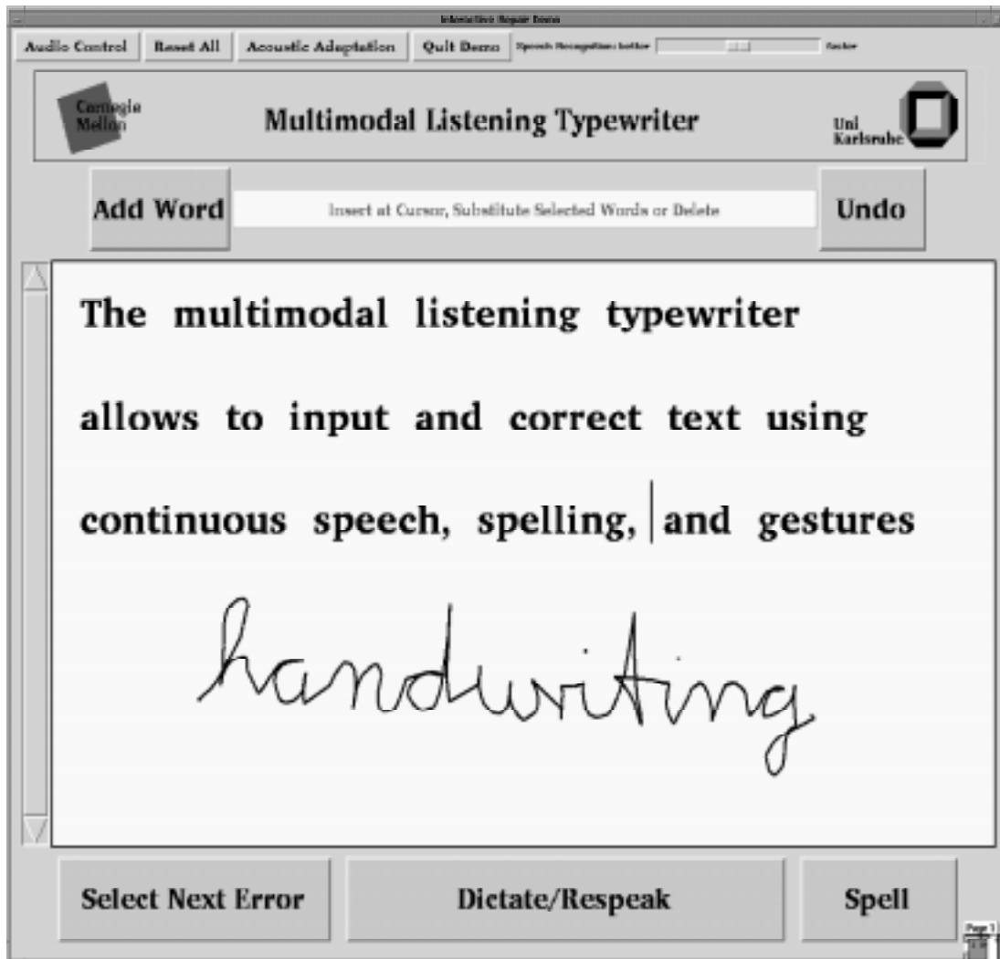
Figure 8. GUI of the prototype multimodal dictation system
