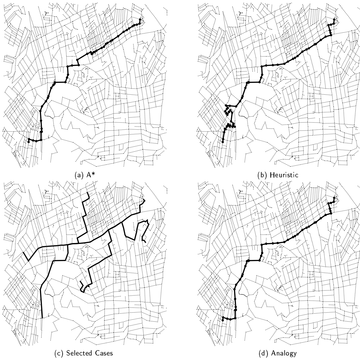
Figure 16: (a) The path generated by A*. (b) The path generated by a search heuristic. (c) The cases selected. (d) The path generated by analogy.
