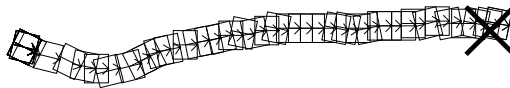
Fig. 3. Sample trace of the execution of the reactive control algorithm. The target point is marked with a cross.
