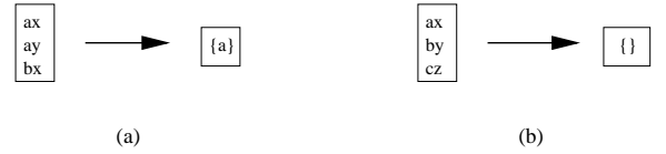
Figure 5: Independent action examples. (a) In this leaf, action a is can be performed independently by agent 1, since it forms an optimal joint action with x and y , all the possible actions that agent 2 might perform at this leaf. (b) There is no Independent action for agent 1 in this leaf.
