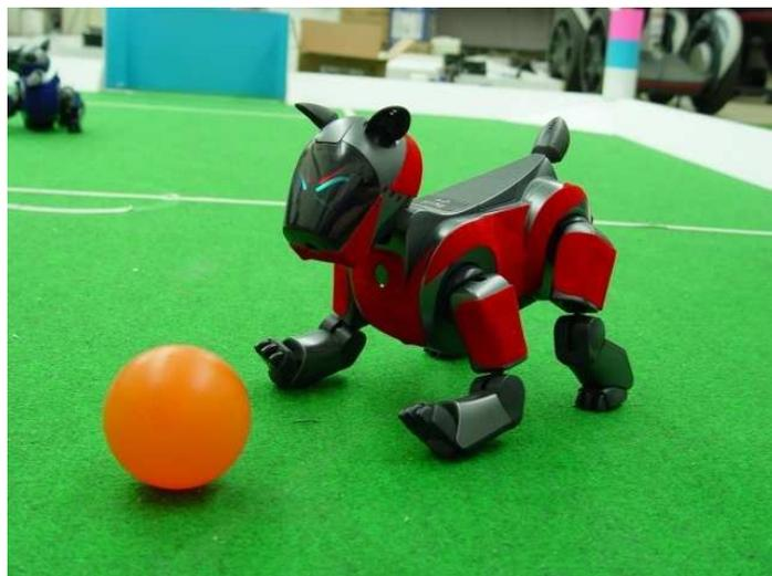
Figure 1: Sony AIBO ERS-210 with a soccer ball.
