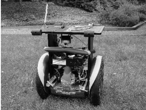
**Figure 1. The Segway RMP robot.**
