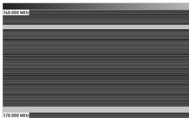
Figure 6. Assignment results for greater Pittsburgh area for a UHF device with 150 channels. Darker bands are assigned, lighter bands are used, light gray is unused. Note logarithmic scale for frequency.
