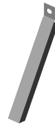
Figure 2.13 – Isometric view of the legs that has the whole being used to mount motor
