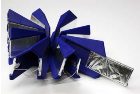
Fig. 5. The electrodes slide into slots on the star shaped face.
