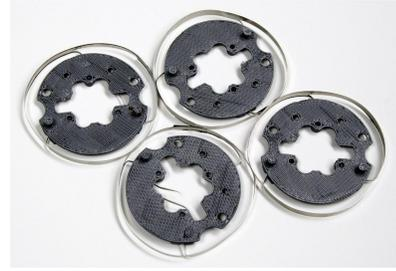
Fig. 7. Using mechanical contacts for power conduction.
