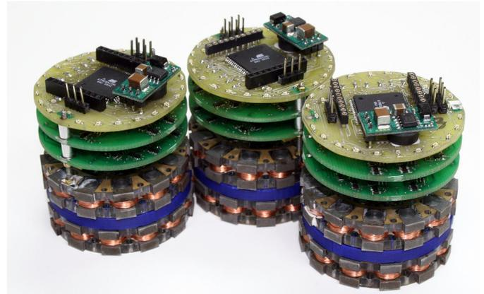
Fig. 1. Three magnetic 45mm planar catoms. Videos demonstrating their movement capabilities are available at <http://www.cs.cmu.edu/~claytronics/iros07/planarcatom/>.
