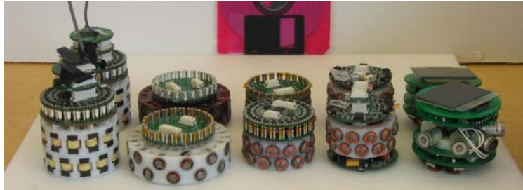
Pairs of Catoms from prototypes 7 through 2 (left to right)
