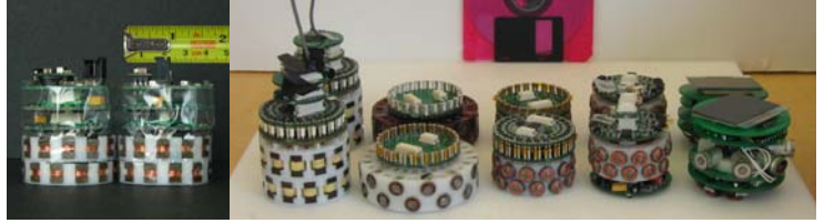
Pairs of Catoms from prototypes 7 through 2 (left to right)
