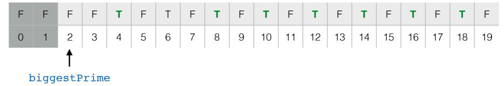
Next time through the outer loop, multiples of 3 will be marked as composite, etc.
