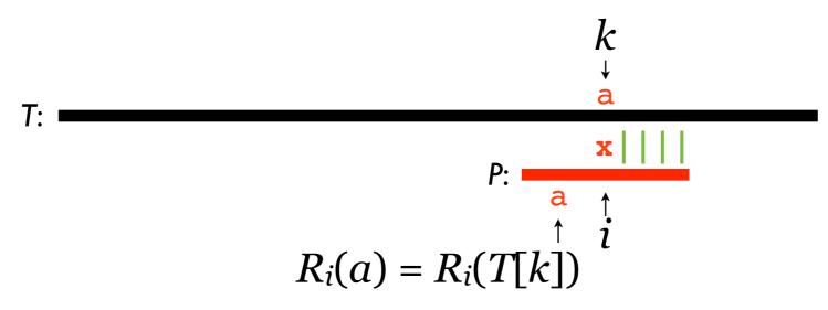
shift by *i* -  $R_i(T[k])$  characters so that the next occurrence of T[k] in the pattern is underneath position *k* in *T*.
