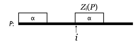
$N_j(P)$  and  $Z_i(P)$  are reverses of each other:  $N_j(P) = Z_{n-j+1}(P^r)$ , where  $P^r$  is P reversed.  $\leftarrow \quad Can \ compute \ in \ O(n) \ time \ using \ Z-algorithm \ on \ P^r$ .
