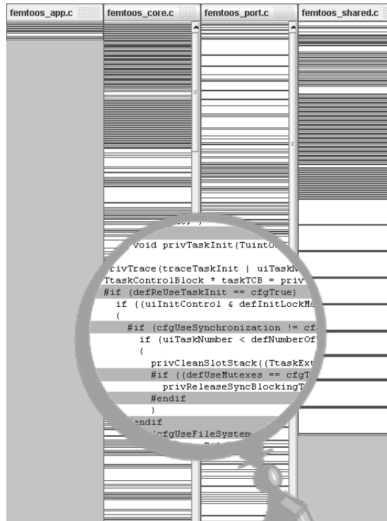
Fig. 2. Preprocessor directives in the code of Femto OS: Black lines represent preprocessor directives such as #ifdef , white lines represent C code, comment lines are not shown [49].
