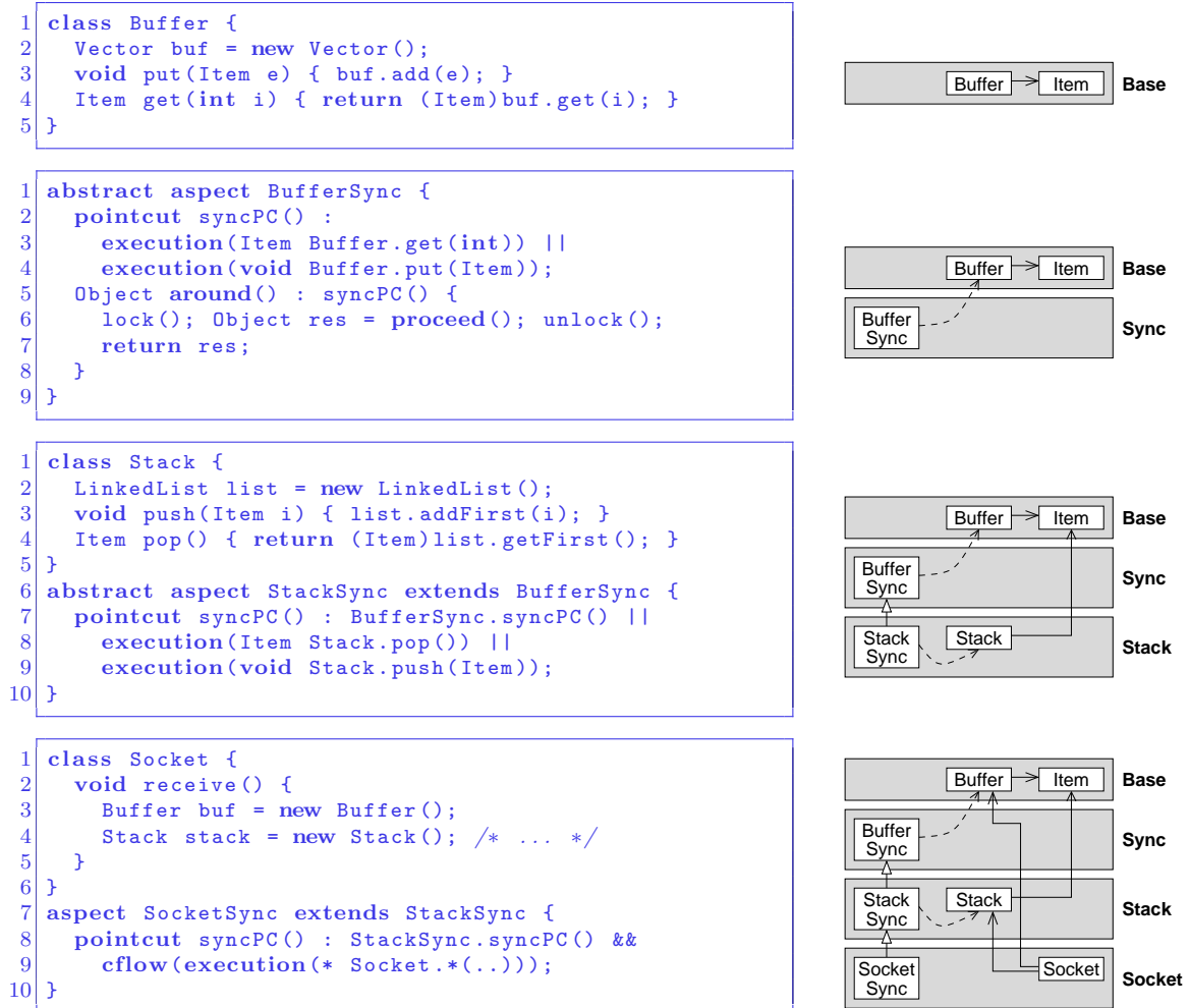
Figure 2: Four steps in the evolution of a program using aspects.
