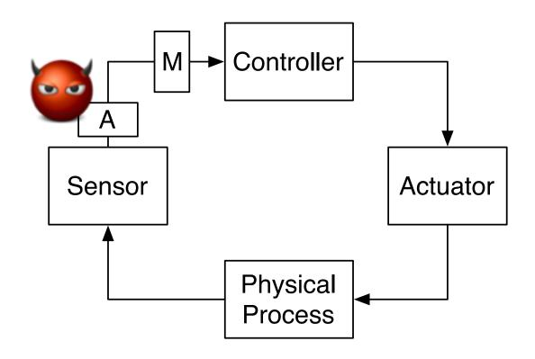
Traditional ICS retrofitted with modern network technology Different failure models in security!
