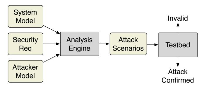
Build formal models of system & attacker (e.g., state machines) Specify security req. using a formal notation (e.g., temporal logic) Analyzer exhaustively explores all possible sequences of attacker actions (model checking)
