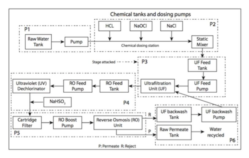
Six different treatment stages (P1 – P6) Each stage monitored by sensors for water quality
