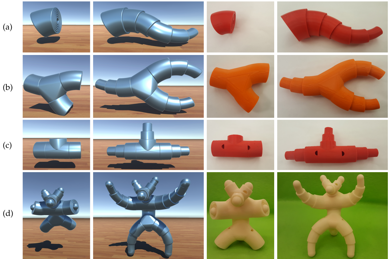
Fig. 12. Left: Telescopes designed using our pipeline. Right: 3D printed physical prototypes.
