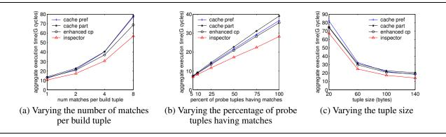
Figure 12: Aggregate total performance varying three parameters when 8 CPUs are used in the join phase
