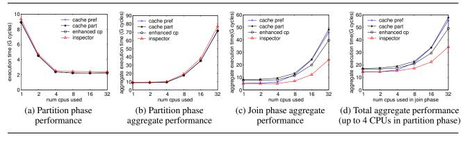
Figure 10: Varying the number of CPUs used
