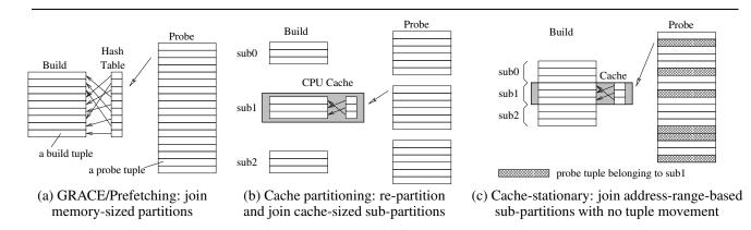
Figure 3: Comparing the cache behaviors of different join phase algorithms
