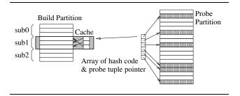
Figure 9: Joining a pair of build and probe sub-partitions
