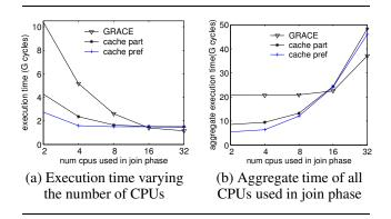
Figure 1: Impact of memory bandwidth sharing on join phase performance in an SMP system
