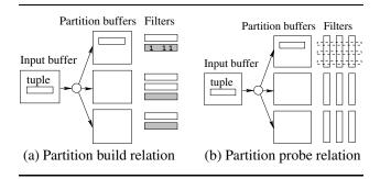
Figure 7: I/O partition algorithm
