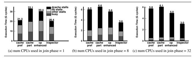
Figure 11: Join phase CPU time breakdowns for CPU 0
