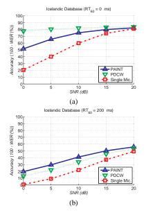
Figure 3: Comparison of speech recognition accuracy using PAINT, PDCW, and the baseline for anechoic environment (Fig. 3a) and for reverberant environment (Fig. 3b) with  $T_{60} = 200ms$ .
