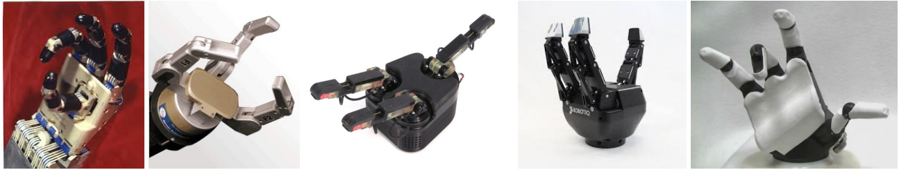
Figure 7: Hands Atkeson has worked with. Note the prevalence of hard surfaces and rigid palms. L-R: Utah/MIT, Barrett, IRobot, Robotiq, and Sandia hands.
