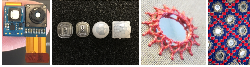
Figure 12: Left: A small time of flight camera. Middle: Front and back view of a lens for an optical mouse, and faceted dome lenses (transparent to infrared). Right: Shisha embroidery, in which mirrors are sewn into fabric. We propose sewing cameras into fabric. Low profile lenses are needed for this approach to whole body vision.
