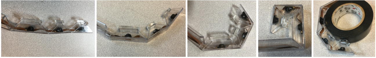
Figure 3: Kinematic prototype of a finger skeleton with cameras.
