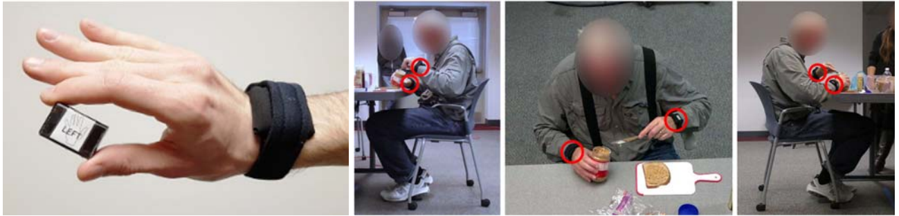
Figure 10: Left: A wearable accelerometer system. Right: A Parkinson's patient whose tremor is being monitored by cameras and wearable accelerometers (red circles).
