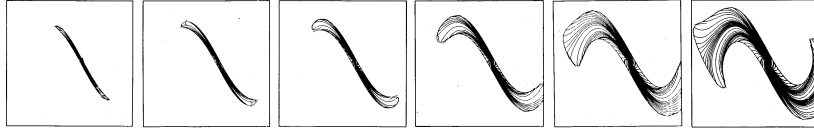
Figure 5: Computing a 1D swingup value function using an adaptive grid.
