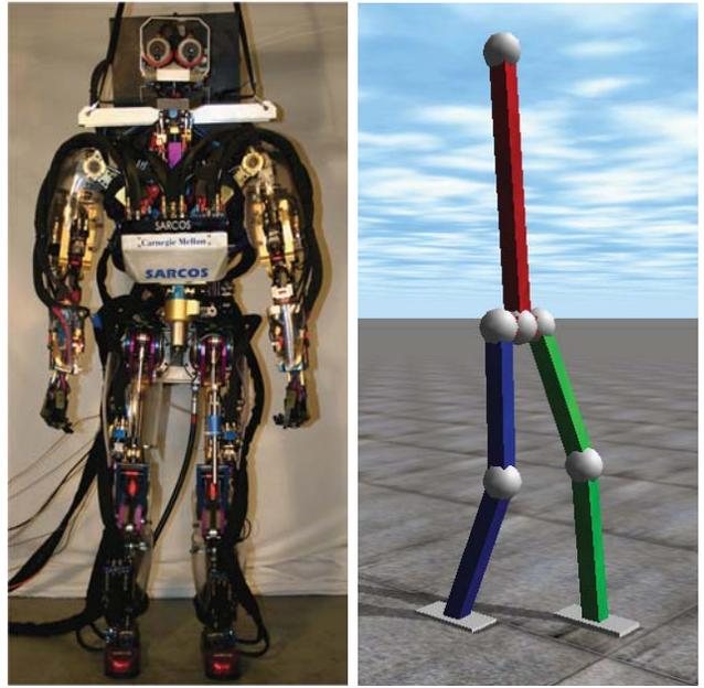
Fig. 1. The Sarcos Primus hydraulic humanoid robot (left) and the simulation based on it (right).
