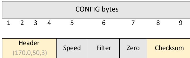
The *Checksum* (UINT16) needs to be calculated according to the value of the Speed, Filter and Zero.
