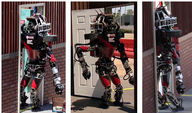
Fig. 1. Successful sidestepping through the door (left, middle) and the failure in the DRC rehearsal (right) in which the protective cage (black padding) for the head is against the white door frame.
